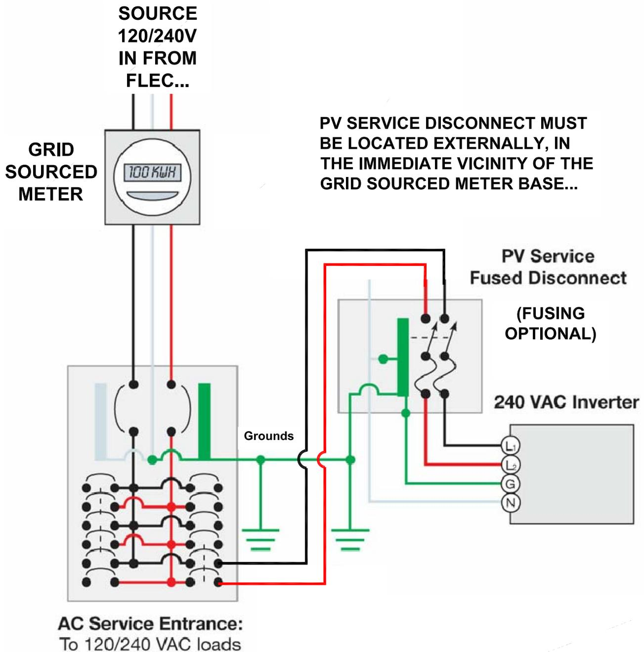
**PV SERVICE DISCONNECT MUST BE LOCATED EXTERNALLY, IN THE IMMEDIATE VICINITY OF THE GRID SOURCED METER BASE...**
